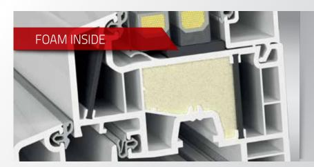
Further improvement of the thermal performance of the window by optionall filling of the chosen internal profile chambers with polyurethane foam, after welding of the window construction.
